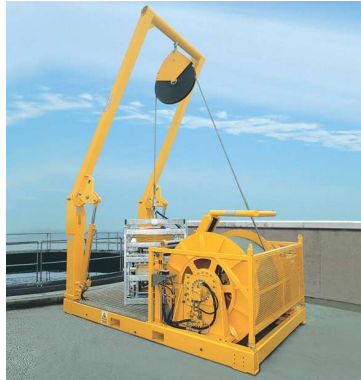
'A' frame erected ready to lift ROV & TMS
