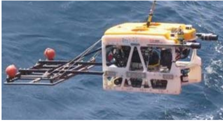
SURVEY SKID WITH TSS PIPE TRACKER
