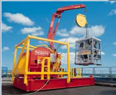
Launch & Recovery System (LARS) & TMS
